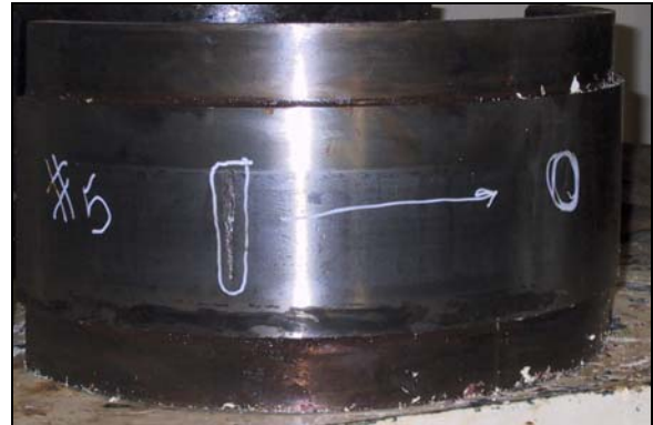
Photo 7 Damaged Race of Roller Bearing
