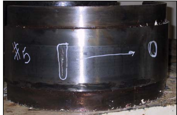
Photo 7 Damaged Race of Roller Bearing
