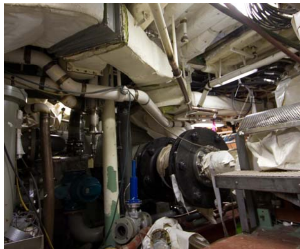
Photo 3 LCS 3 AMR Gear Coupling Shaft Flex Coupling
