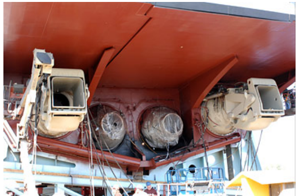
Photo 8 Steerable and Fixed Waterjets
