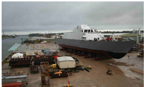
Photo 9 Rolling Hull to Launch Ways
