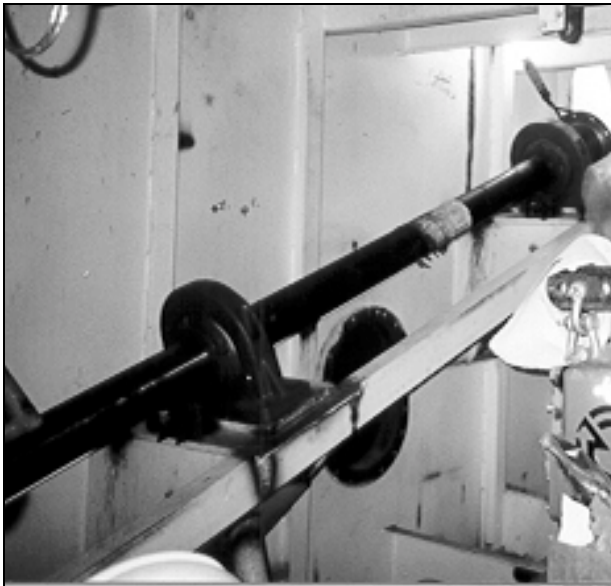
Photo 5 Modified Bearing Supports: Case 3
