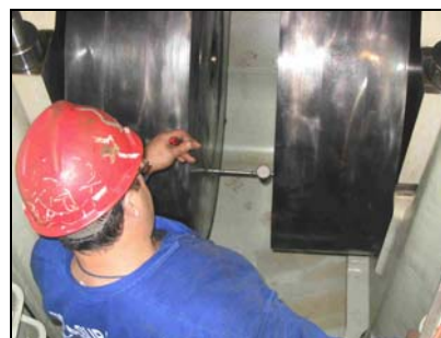
Figure 3 Crankshaft Web Deflection Measurements
