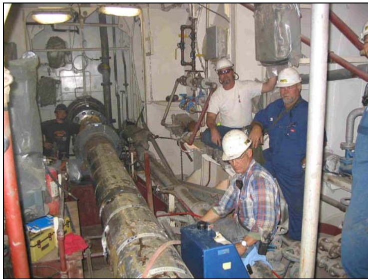
Figure 11 Alignment Measurements on Lineshaft: MV Jean Anne
