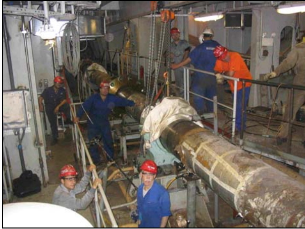
Figure 6 Jack Up Load Tests on Lineshaft
