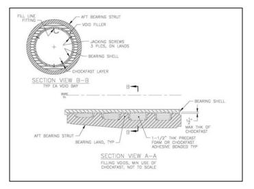
Figure 4 - Chocking Arrangement - Initial Concept
