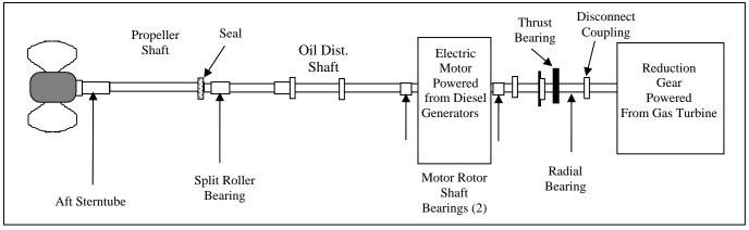
Figure 1 - Schematic of Center Shaft
