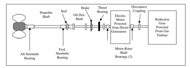
Figure 2 - Schematic of Wing Shaft
