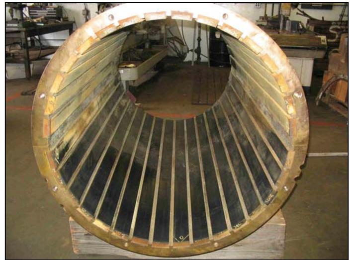
Photo 7 - Forward Sterntube Bearing - Looking Aft
