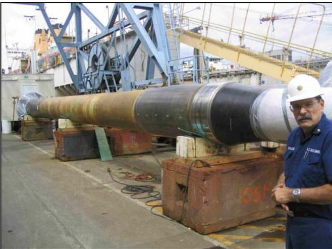
Photo 3 – Wing Propeller Shaft
