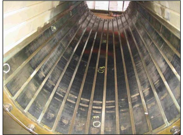
Photo 6 - Aft Sterntube Bearing - Looking Aft
