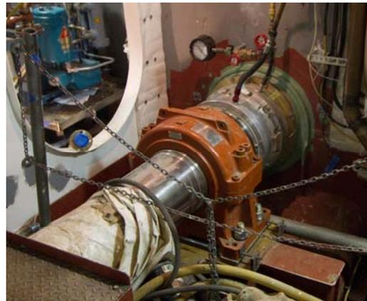
**Photo 2 LCS 3 Port Boost Waterjet Lineshaft, Bearing and Seal**
