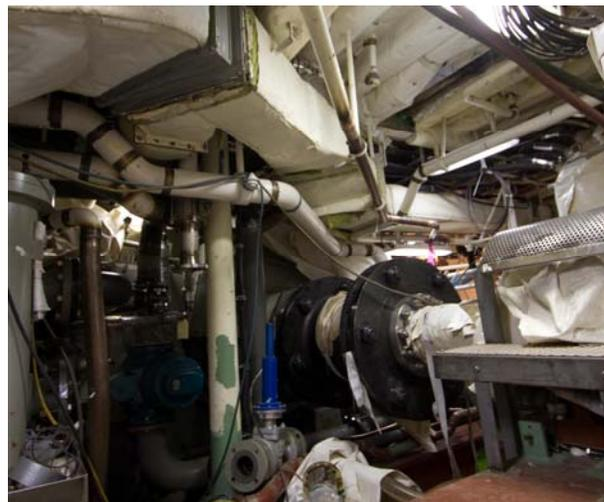
**Photo 3 LCS 3 AMR Gear Coupling Shaft Flex Coupling**
