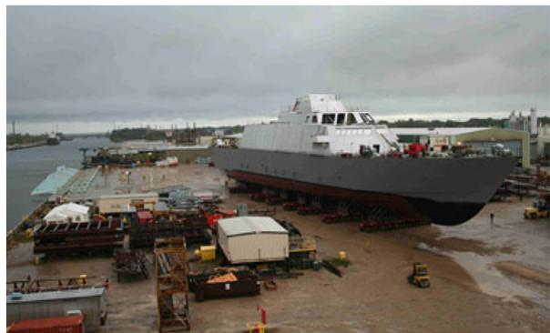
**Photo 9** Rolling Hull to Launch Ways
