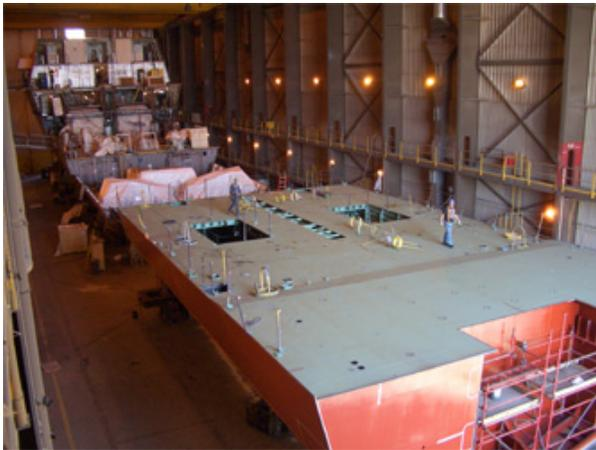
**Photo 5** Hull Under Construction
