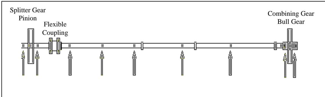
**Figure 2 Gear Coupling Shaft Finite Element Model**
